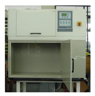
Two bars are provided on left and right side of the test chamber bottom to allow the use of standard specimen tray. It is easy to remove the 2 bars for maximum aperture of the chamber bottom.
