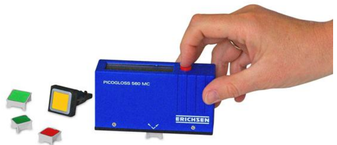
PICOGLOSS 560 MC-S – Gloss measurement on small specimens
